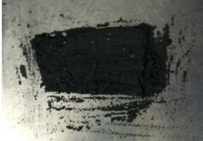
Figure 3: Copper Oxide /Aluminum Powder mixture (Thermite)
